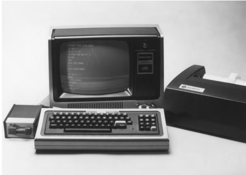
Figure 7.1 The Tandy TRS-80 microcomputer with video display, keyboard, Exatron printer, and a disk device. This system was popular among early hackers and self-taught programmers, and it featured a popular adaptation of BASIC. (Courtesy of the Computer History Museum)
