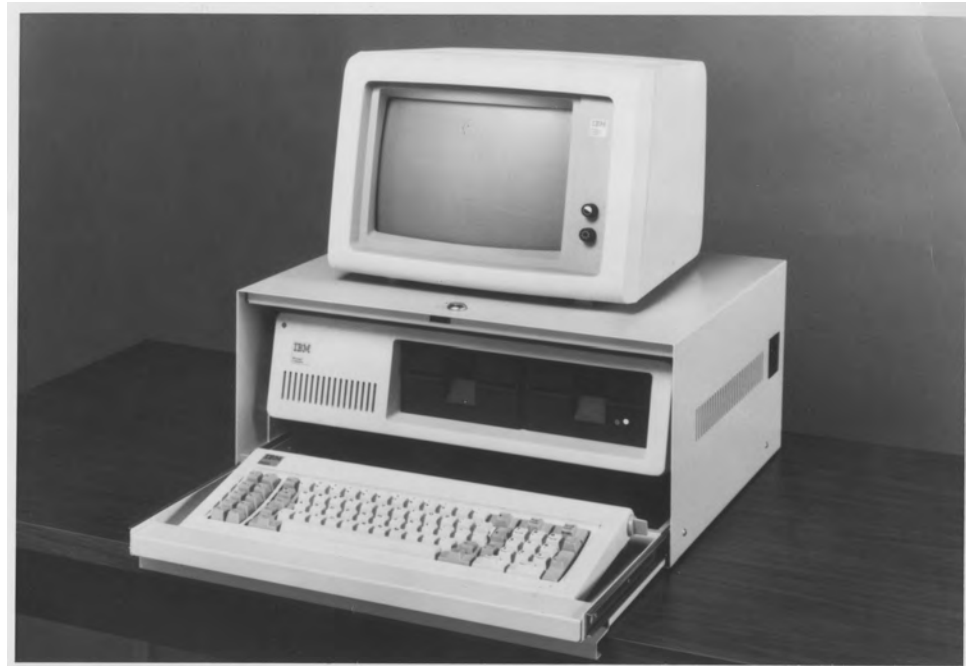
Figure 7.2 An original IBM Personal Computer (1981) with the Mead-Hatcher Inc.'s locking “Fortress” cabinet, designed to secure a PC from unauthorized entry. In the early years of personal computing, securing a computer physically was considered an appropriate way to protect the device from unauthorized use. (Courtesy of the Computer History Museum)
