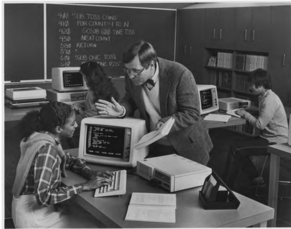
Figure 5.6 Designed for the home and educational market, the PCjr featured a “Cartridge BASIC” version of the BASIC interpreter that could be inserted as firmware into one of the two slots on the front of the desktop computer. This staged image from 1984 depicts children learning BASIC at school. A short BASIC program that simulates coin tosses appears on the chalkboard. (Courtesy of the Computer History Museum)
