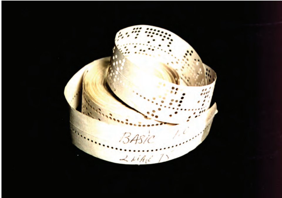
Figure 3.1 Photograph of the punched paper tape for MITS Altair BASIC 1.0, created by Bill Gates, Paul Allen, and Monte Davidoff for the Altair 8800 microcomputer. Dated March 2, 1975. (Courtesy of the Computer History Museum)
