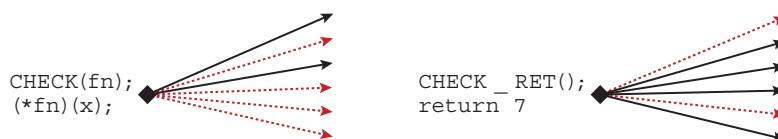
Figure 1.2 A CFI mechanism restricts control-flow hijacking to targets that are valid according to a pre-determined control-flow graph (black arrows). All other targets are rejected (red arrows).
