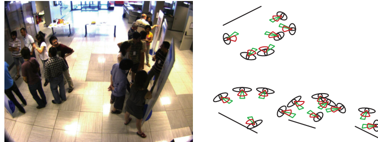
Figure 3.5 Frame example: (left) the original image of one of the cameras, (right) the head–green and body–red pose estimates plot in bird’s-eye view.
