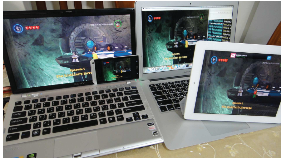
Figure 11.2 Demonstration of a running GamingAnywhere system. There are four devices in the photo: one game server (the left-hand side laptop) and three game clients (a MacBook, an Android phone, and an iPad 2). (Adapted from Huang et al. [2013a]) (LEGO Batman software is copyrighted by Traveller's Tales Games Publishing Ltd.)
