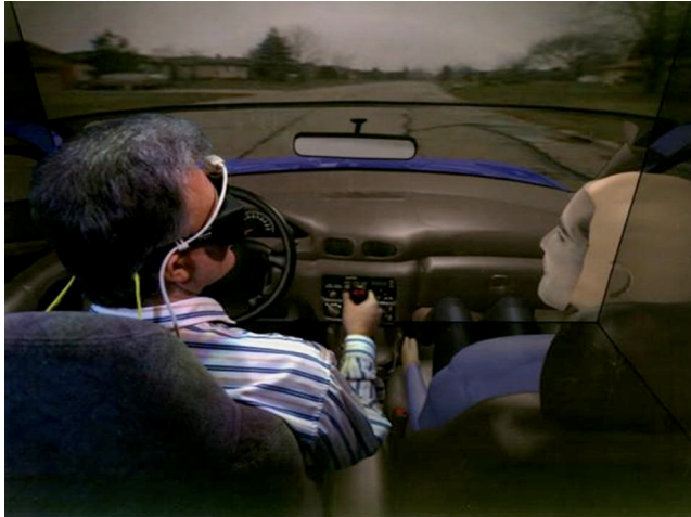
Figure 22.4 A user drives a virtual car in a CAVE while speaking with an avatar controlled by a remote user. (From Daily et al. [2000])
