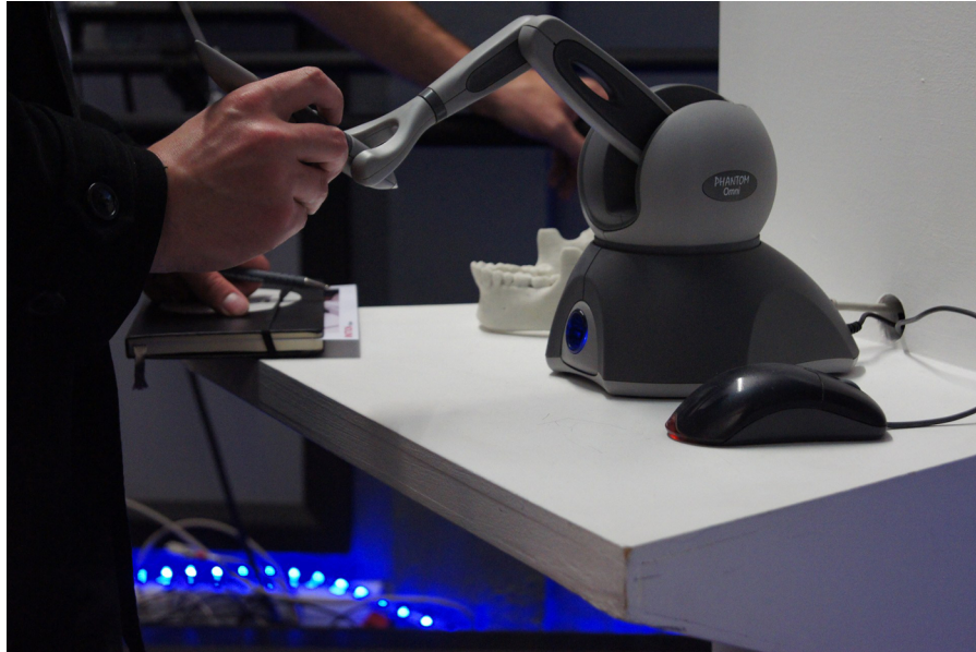
Figure 3.11 Sensable's Phantom haptics system. (Courtesy of INITION)
