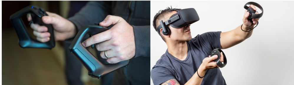
Figure 27.3 The Sixense STEM (left) and Oculus Touch (right) tracked hand-held controllers. (Courtesy of Sixense (left) and Oculus (right))
