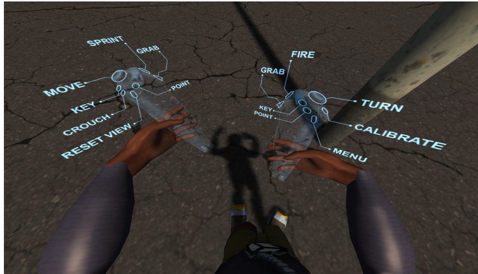
Figure 26.3 A simple transparent texture in the hand can convey the physical interface. (Courtesy of NextGen Interactions)
