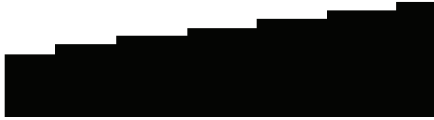
Figure 21.2 Jaggies/staircasing as seen on a display that represents the edge of an object. Such artifacts result due to discrete sampling of the object.
