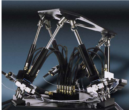
Figure 3.13 An active motion platform that moves via hydraulic actuators. A chair can be attached to the top of the platform. (Courtesy of Shifz, Syntharturialist Art Association)
