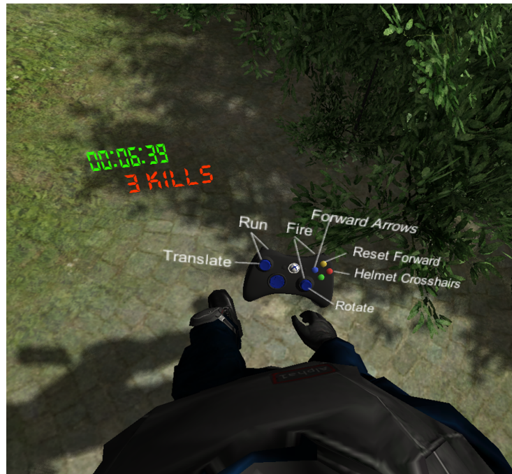
Figure 26.2 Information and a visual representation of a non-tracked hand-held controller in the torso reference frame. (Courtesy of NextGen Interactions)
