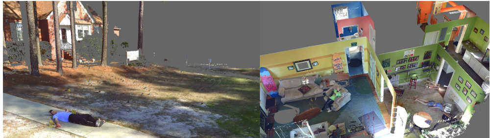
Figure 21.7 Mock crime scenes captured with a 3rdTech laser scanner. Even though artifacts such as cracks and shadows can be seen in parts of the scene that the laser scanner(s) could not see (e.g., behind the victim’s legs), the results can be quite compelling. (Courtesy of 3rdTech)
